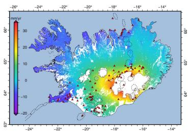
Estimated average vertical velocities induced by GIA between summer 2015 and summer 2020 in Iceland, derived from Sentinel-1 interferometry, using the procedure described by Drouin and Sigmundsson (2019).
